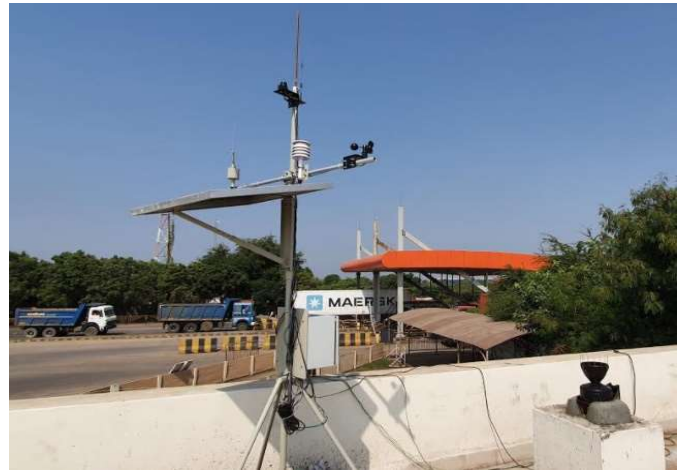
Micro Meteorological Station at Port
